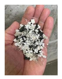
More than 30,000 tons of polystyrene is used as packaging, in SA, on an annual basis. Upcycling this waste into energy efficient floor and walling products means diverting waste from landfill whilst also presenting a new, distinctive way of building.
