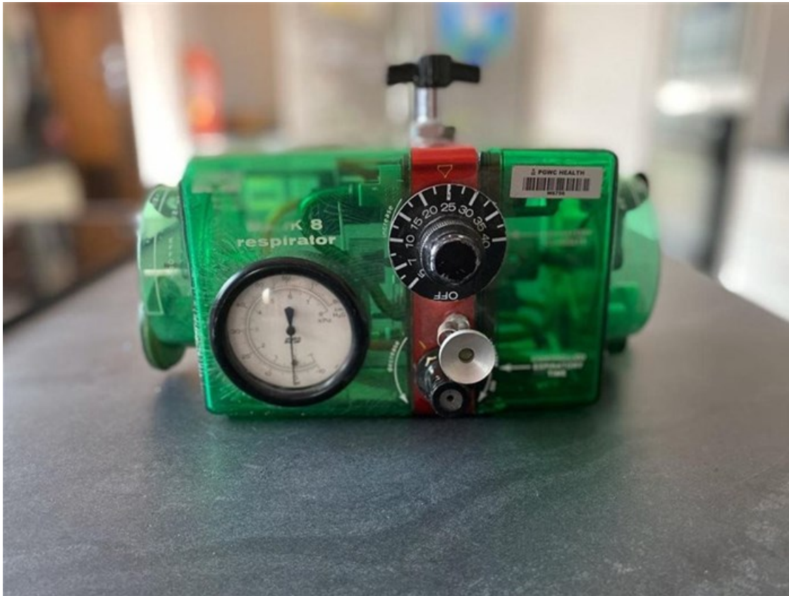
An existing mechanical respirator being reverse-engineered to be used as an emergency ventilator.
